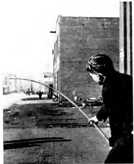
Whip test of a 20-foot welded brass tube made up of an 8 and a 12-foot length.
